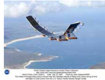
Unmanned Helios Aerovironment 30'000 m, 21 KW
